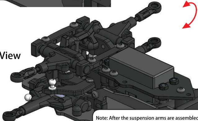
Note: After the suspension arms are assembled, they should be able to move up and down freely.
