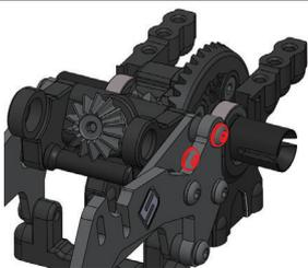
Note: M3 x 10mm & M3 x 18mm Button Screw (4pcs) does not need to be tightened as shown in the above diagram.
