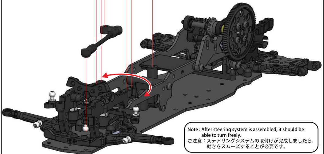
Note: After steering system is assembled, it should be able to turn freely.
